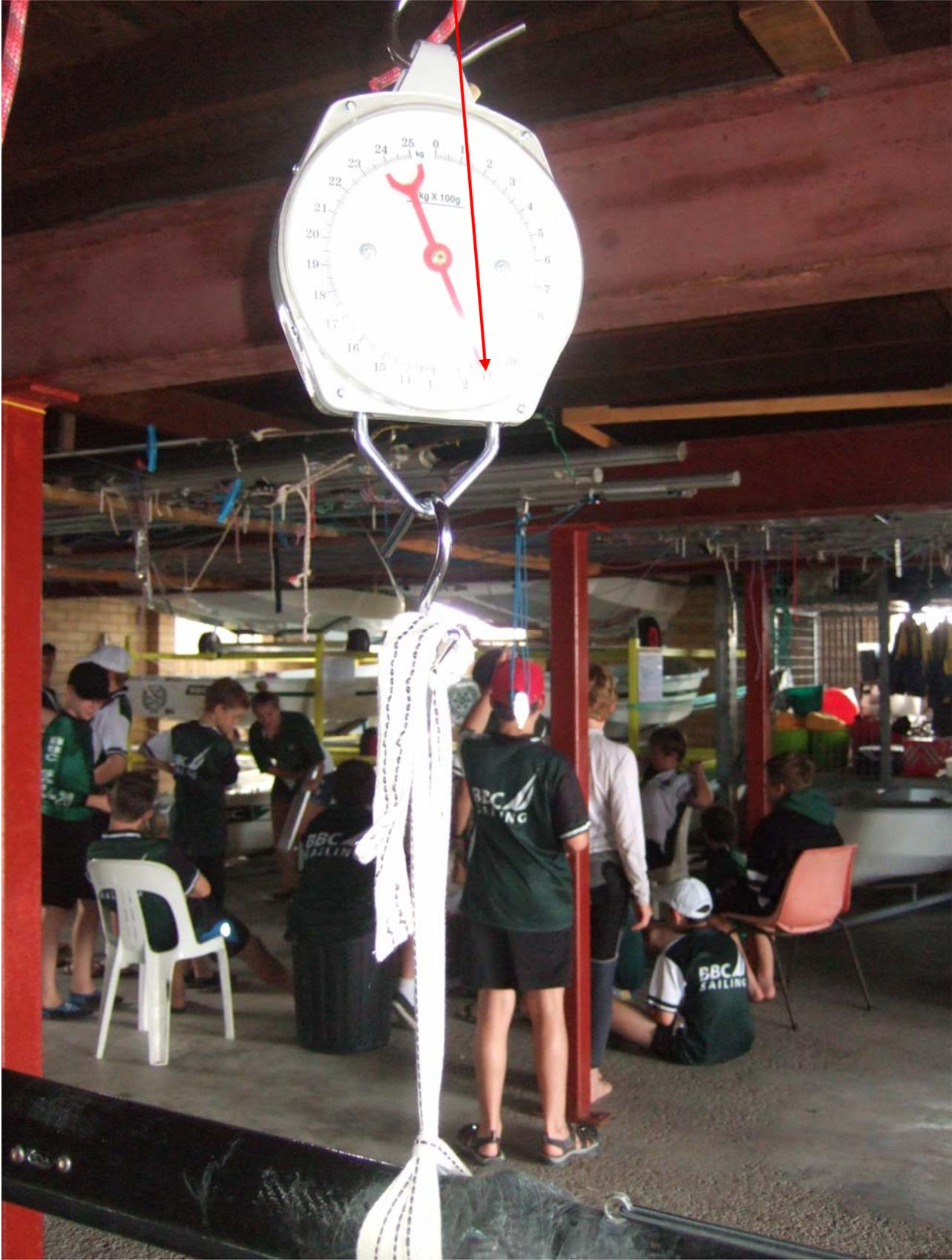
**PHOTO No4** (check mast balance point is at, or above, 42% marker)
