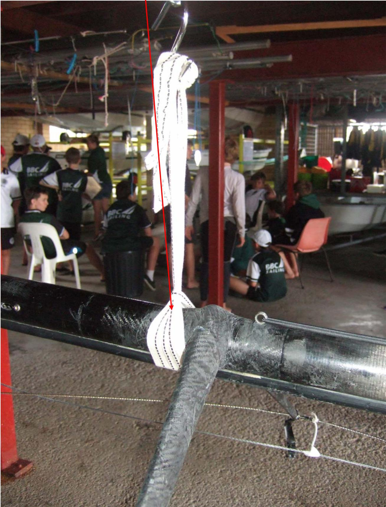
**PHOTO No3** (check weight – minimum 11kg for No1 mast and 10kgs for No2 mast)
